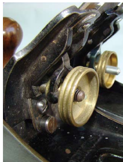
Minor adjustments – The frog adjustment screw, just below the brass adjustment knob permits a degree of back-and-forth positioning.
