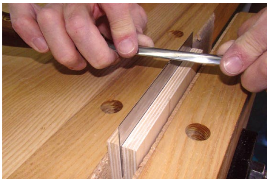
Heavy hand be gone – Burnishing a hook on a scraper needs only a few light strokes with the burnisher held at an angle of about five or 10°.
