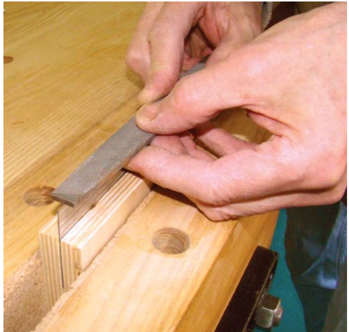
Joint your edges – You must take care to keep the file square to the scraper if you are doing this freehand.
