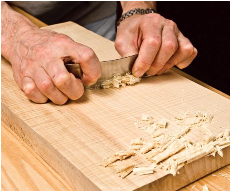
Shavings not dust – A properly prepared card scraper will produce gossamer-thin shavings in the most difficult of woods.
