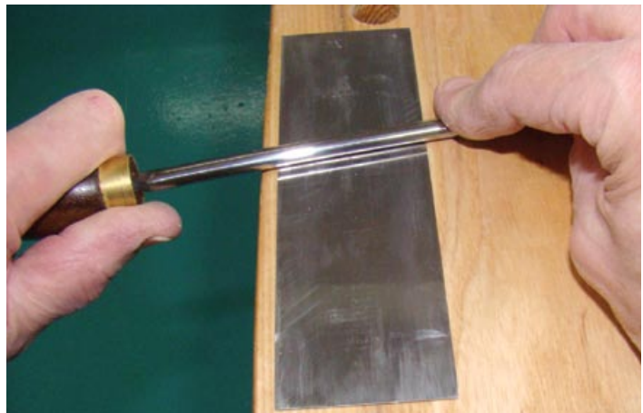
Work the steel – Several strokes by the burnisher held flat against the scraper's face work-hardens the metal while forming the beginning of a hook.
