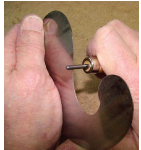
Throwing a curve – Burnishing the hook onto a curved scraper is much like using a paring knife to peel a potato.
