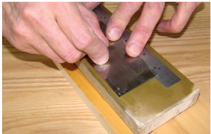
Ruler trick it – By supporting one edge of your scraper on a thin steel ruler, you'll only have to hone a small section of the scraper's face.
